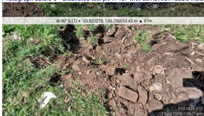
Photograph 11.1.1-6 Excavated test pit TP467 with demolition rubble including ACMs
